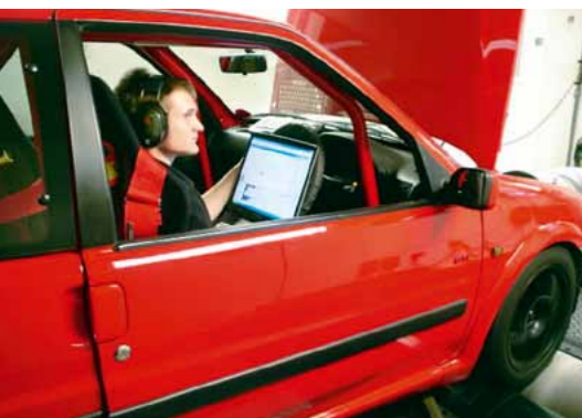
The new minimum TPS value is now entered into the ECU and Idle controls switched back on.
